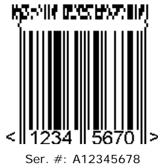
Figure 5.9.8-3. EAN-8 symbol with a three-column CC-A
