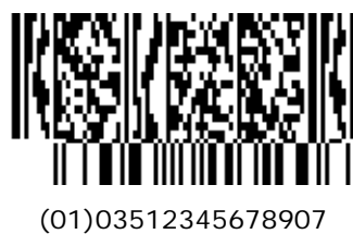
Figure 5.9.8-7. GS1 DataBar Limited symbol with a three-column CC-B
