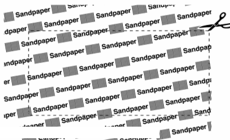
Figure 6.3.3.7-2. Barcode placement on random-wrapped item
