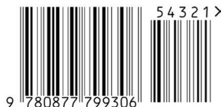
Figure 5.2.2.5.2-2. EAN-13 barcode with five-digit add-on symbol
