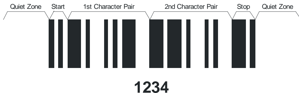
Figure 5.3.2.1.2-2. ITF-14 symbol inclusive of Quiet Zones
