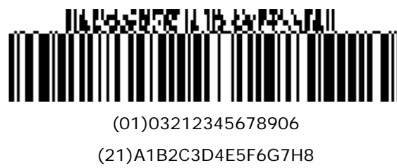
Figure 5.9.8-9. GS1-128 symbol with a four-column CC-A
