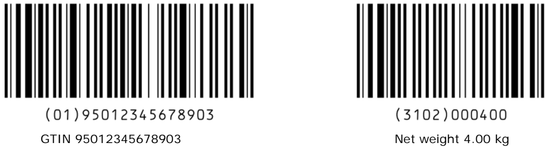
Figure 7.8.5.1-2. Data encoded in one concatenated GS1-128 symbol
