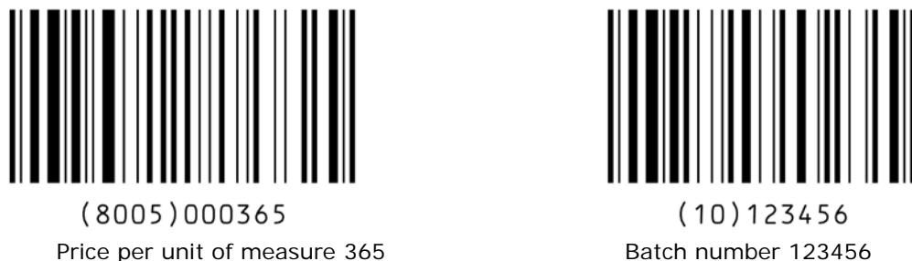
Figure 7.8.5.2-1. Data encoded in two GS1-128 symbols
