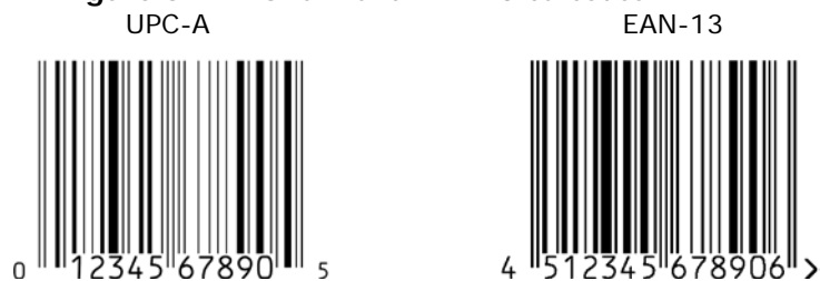
Figure 5.1-1. UPC-A and EAN-13 barcodes
