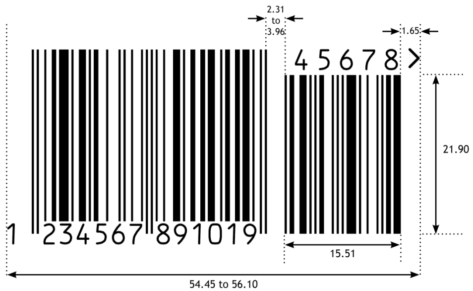
Figure 5.2.6.6-6. EAN-13 barcode with five-digit add-on symbol
