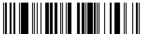
Figure 5.5.2.3.1-1. GS1 DataBar Expanded barcode
