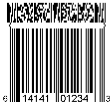
Figure 5.9.8-2. UPC-A symbol with a four-column CC-B component
