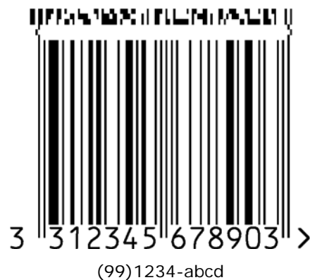
Figure 5.9.8-1. EAN-13 symbol with a four-column CC-A component
