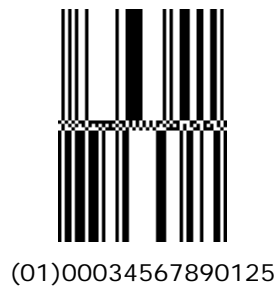
Figure 5.5.2.1.4-1. GS1 DataBar Stacked Omnidirectional barcode
