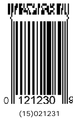
Figure 5.9.8-4. UPC-E symbol with a two-column CC-A
