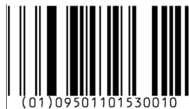
Figure 5.5.2.1.1-1. GS1 DataBar Omnidirectional barcode
