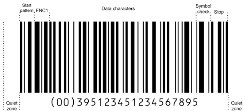
Figure 5.4.2-1. General format of a GS1-128 barcode
